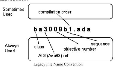
In multiple file tests, the intended order of compilation is indicated by a numeral at position 8. The first file to be compiled has '0', the second has '1', and so forth.
